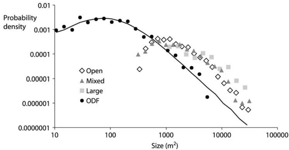
**Figure 8.** Landslide size distributions, given in probability density ((number in bin/total number)/bin width), for each forest cover class in the Siuslaw inventory and for all landslides in the ODF inventory. Solid line shows a double Pareto distribution, equation (15), fit to the ODF data.
