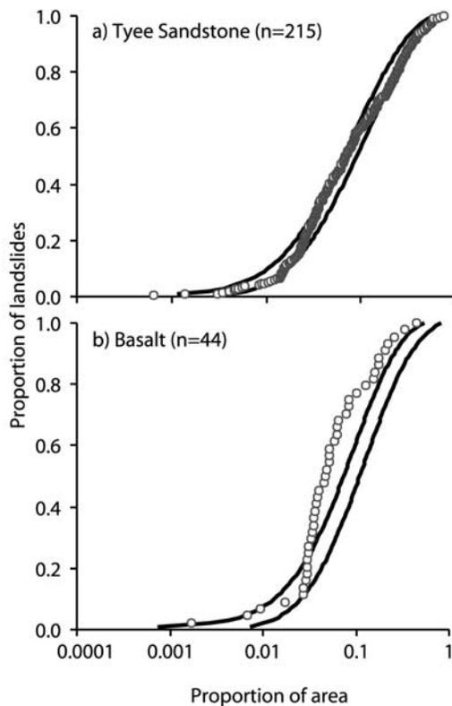
**Figure 6.** Landslide number versus area curves for the ODF field sites separated by rock type: (a) sandstones and (b) basalts. Heavy lines show 90% confidence obtained with Monte Carlo modeling. Open dots are from mapped landslide initiation point locations.
