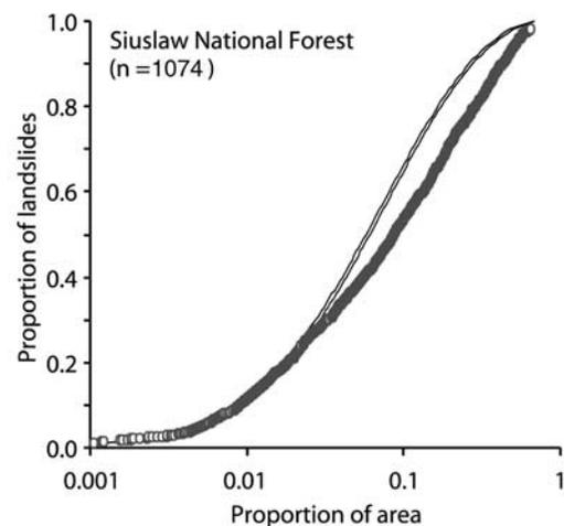
**Figure 7.** Landslide number versus area curves for the Siuslaw National Forest landslide inventory. Solid lines show 90% confidence intervals obtained with Monte Carlo modeling using the topographic weighting term (Figure 3) obtained from the ODF field sites. Open dots from mapped landslide initiation point locations.
