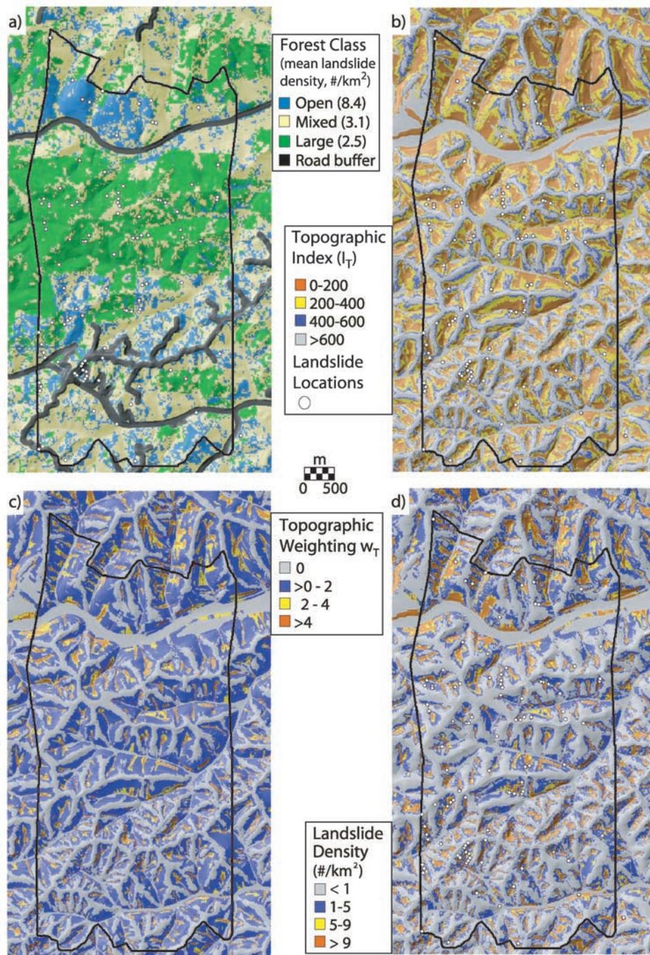
**Figure 4.** Maps from the ODF Mapleton study site showing the (a) topographic and land cover context for field-mapped landslides, (b) topographic index ( $I_T$ ), (c) topographic weighting term ( $w_T$ ), and (d) density of landslide initiation points calculated as the product of the topographic weighting term and the mean landslide density. Study site boundary is indicated by the heavy black line.
