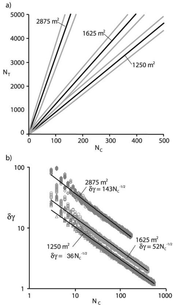
**Figure 9.** (a) Total number of landslides  $N_T$  (black lines), with 90% confidence intervals (gray lines), versus the number counted  $N_C$  based on sampling with replacement from the ODF landslide inventory for three visibility thresholds and (b) width of the 90% confidence intervals for  $\gamma$ , the ratio  $N_T/N_C$ , for each of these thresholds.
